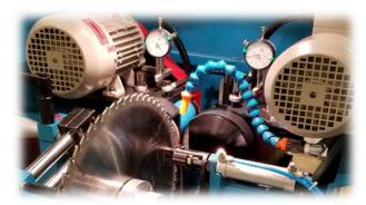
Model BSG-32K: Manual side grinder for carbide tipped saw blades
