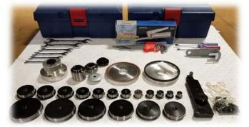
All machines come with a complete set of tools, bushings, one set of grinding wheels and startup machine fluids.
