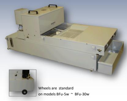
All of our standard BF $\mu$ -Series filters are equipped with a filterable coolant pump, one roll of filter media and chip collector. A float switch will automatically activate new filter media as required.
